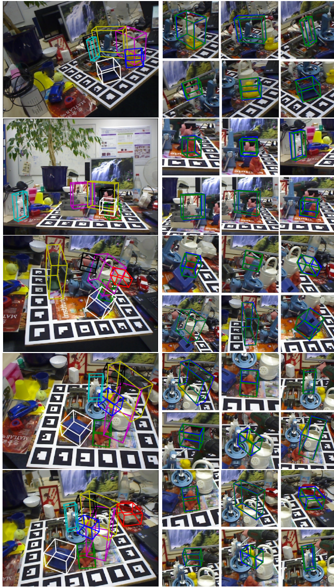
Figure 7: Qualitative 6D pose estimation results on the OCCLUSION dataset. We only draw the 3D bounding boxes rendered by predicted poses. Our approach is robust to partial occlusion and illuminations.
