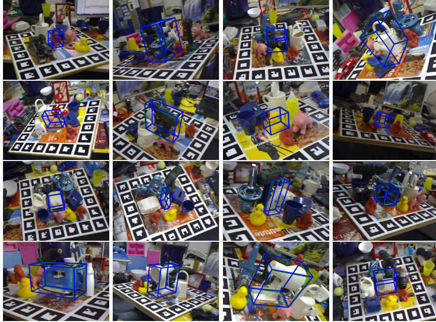
Figure 5: Qualitative 6D pose estimation results on the LINEMOD dataset. The green and blue bounding boxes are rendered using ground truth poses and predicted poses, respectively. As can be seen, our method is robust to scale and light changes.
