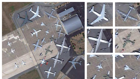
Fig. 1. Aircraft examples with intraclass variation. Examples at right columns show that intraclass variation is derived from aircraft type, rotation, and size.
