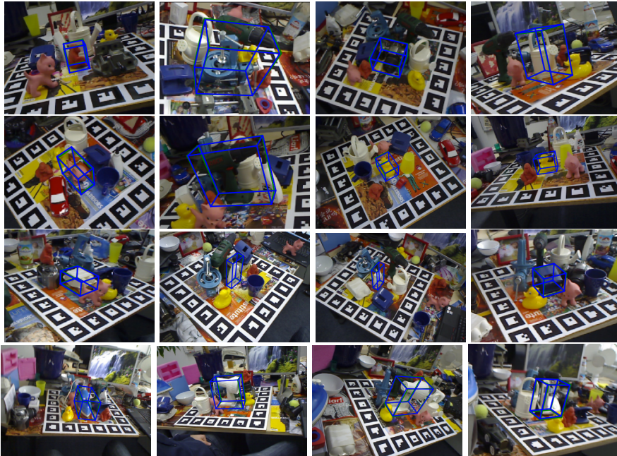
Figure 4: We present qualitative 6D pose estimation results on the LINEMOD dataset. The green and blue 3D bounding boxes are rendered using ground truth poses and predicted poses, respectively.
