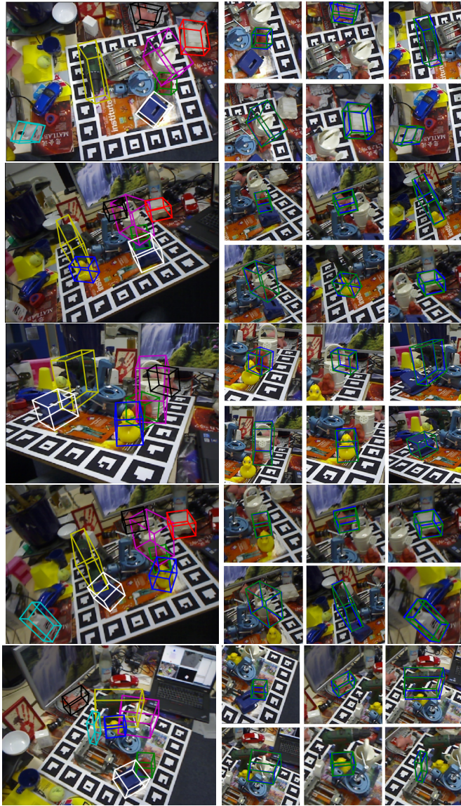
Figure 5: We present qualitative 6D pose estimation results on the OCCLUSION dataset. In left column we only draw the 3D bounding boxes rendered by predicted poses. In right column we render the green and blue 3D bounding boxes using ground truth poses and predicted poses, respectively.
